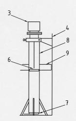
a) Installation of top-mounted ALGs on fixed-roof tanks with still-well
