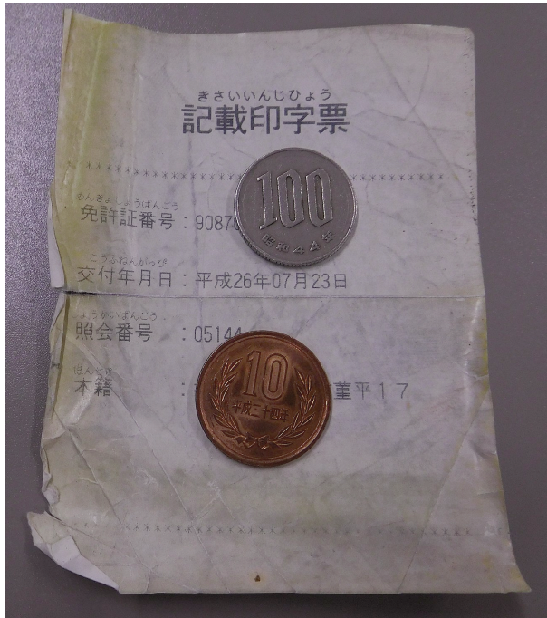
“Durable proof”: Thermoprinted receipt, which can become hard to read over time
