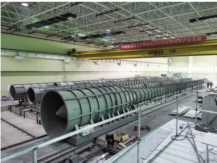
Figure 2: The primary stack flowrate calibration facility
