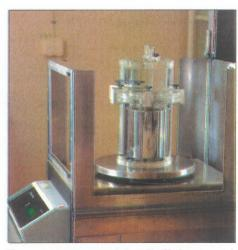
Fig. 4 The pycnometer, containing distilled water and the test weight, is weighed on a high accuracy nonautomatic weighing instrument.
