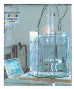
Fig. 3 Sophisticated equipment for highest accuracy density determination
