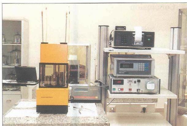
Fig. 5 The 1 kg mass comparator with air buoyancy artefacts
