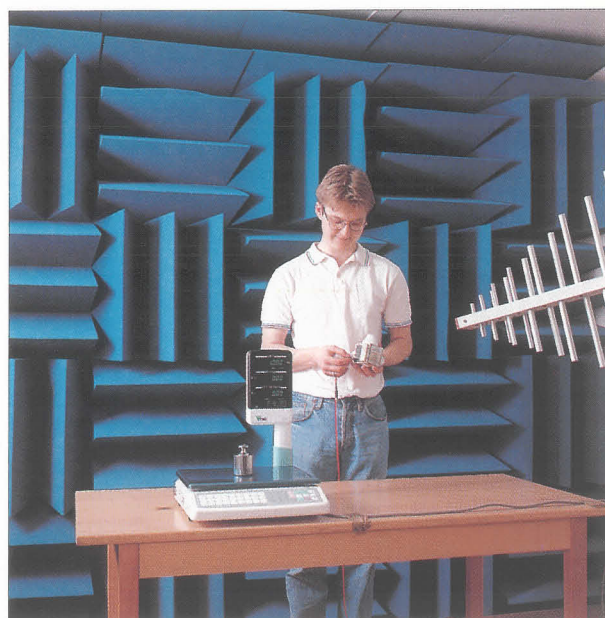
Fig. 1 Testing immunity to radiated electromagnetic fields. The instrument is placed on a wooden table and illuminated by the antenna. A field sensor with an optical fiber cable is installed by the test engineer. The wall is covered with absorbers to minimize reflections of the radiation.
