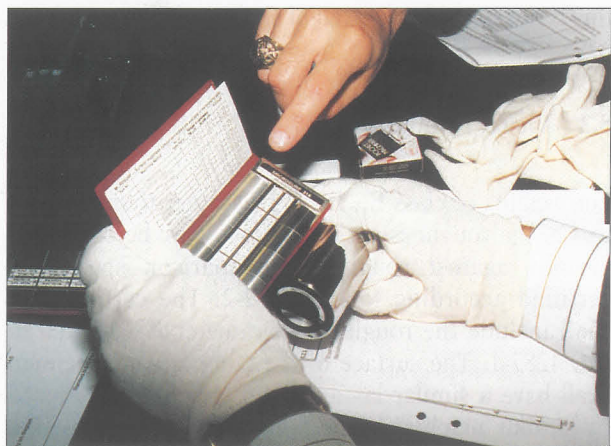
Fig. 3 Surface roughness - visual comparison of an OIML class E 2 weight against a specimen certified according to ISO 2632-2
