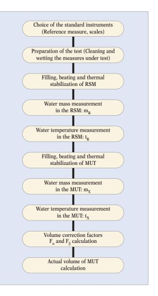
Figure 1 Indirect gravimetric method procedure
