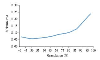
Fig. 4 Influence of grinding granulation of the sample over moisture for soybeans
