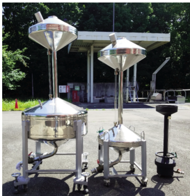
Figure 8 Standard tanks used in the experiment (from left to right: 200 L, 50 L and 5 L)
