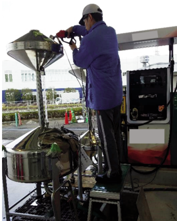
Figure 9 The experiment being conducted. The test liquid delivered from the fuel dispenser under test is being poured into the standard tank.
