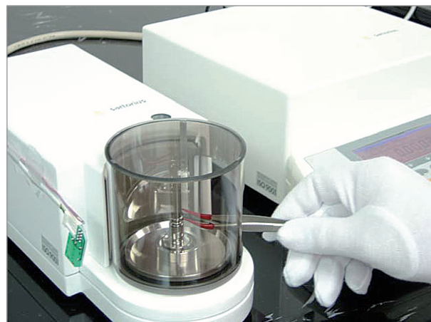
Single substitution on a 10 g – mass comparator of d = 0.1 \mu\text{g}
