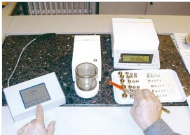
Micro scale with 6 g maximum and scale controller
