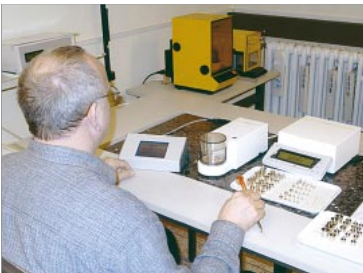
Micro scale with 6 g maximum for the determination of weights of accuracy class E_2
