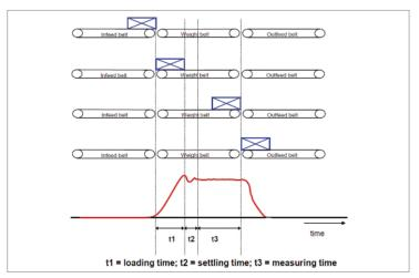
Figure 10 Progression of the measurement signal during movement of a package across the conveyor belts
