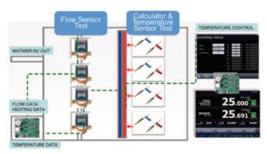
Figure 2 Components of the portable test equipment for a heat meter
