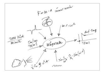
Figure 11 Influences on the weighing sensor (load cell)
