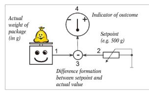
Figure 2 Operating principle of an ACW.
