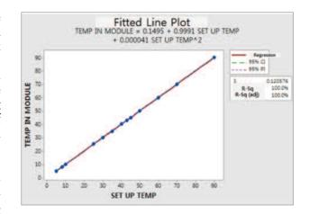
a) Regression line of setup temperature and temperature in the module
