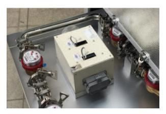
Figure 4 Temperature generation apparatus
