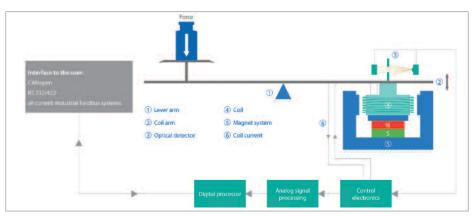
Figure 8 Operating principle of a weighing sensor with force compensation
