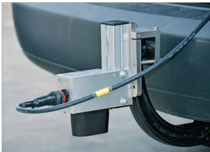
Figure 3 Optical correlator mounted on the METAS vehicle
