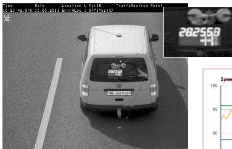
Figure 5 Photo of the METAS vehicle taken by a gate with zoom of the chronometer
