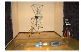
Figure 3 Inside the anechoic chamber with a table for the EUT and an antenna
