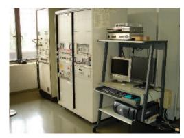
Figure 4 Control system of the renovated electromagnetic environment test facility (NMIJ)
