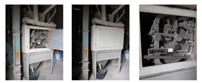
Chronos G 100 at the Demeter Biohof in Hennef-Dambroich (100 kg damping weight). Note that when closed (center picture) it can be locked by key to protect against unauthorized intervention.
