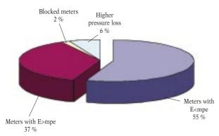
Fig. 2 Verification results of a sample from a batch of gas meters
