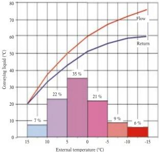
Fig. 4 Typical heat distribution chart
