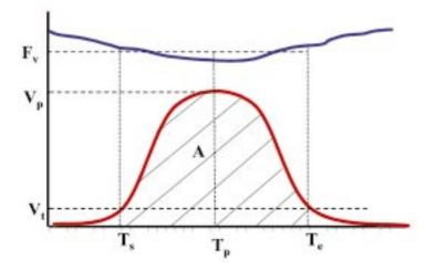
Figure 2 Example of signals measured by WIM-sensor (red) and vehicle (blue). Note: both lines in Figure 2 are examples to explain the measurement principle and not actual measurement signals.
