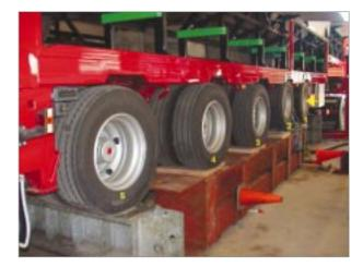
Figure 12 Leveled semi-trailer in the Lab for calibrating the measurement system
