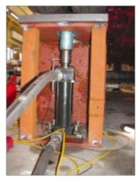
Figure 11 Hydraulic cylinders underneath the first axle
