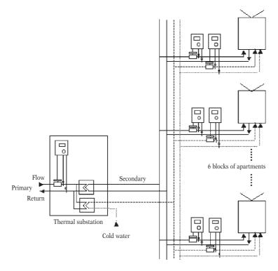
Fig. 3 Solution to meter heat and warm water at blocks of apartments
