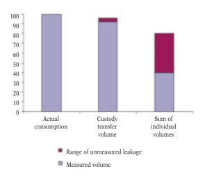
Fig. 1 Water balance in a block of apartments
