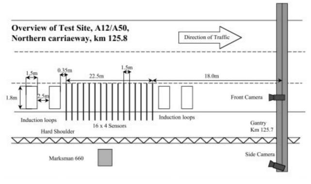
Figure 1 The WIM-Hand test system
