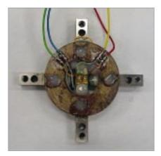
Figure 7 Set of mechanical strain amplifiers in a full bridge set-up
