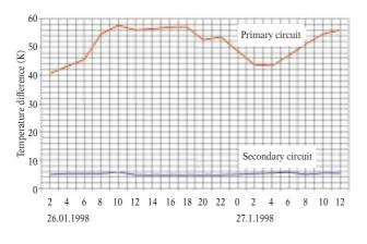
Fig. 5 Comparison between temperature differences in both primary and secondary circuits
