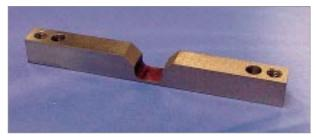
Figure 6 Mechanical stress/strain amplifier
