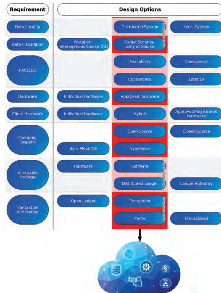
Fig. 4 All design options we identified and the choices we made (red bar). Dependencies among decisions are indicated by a chain linking the items.
