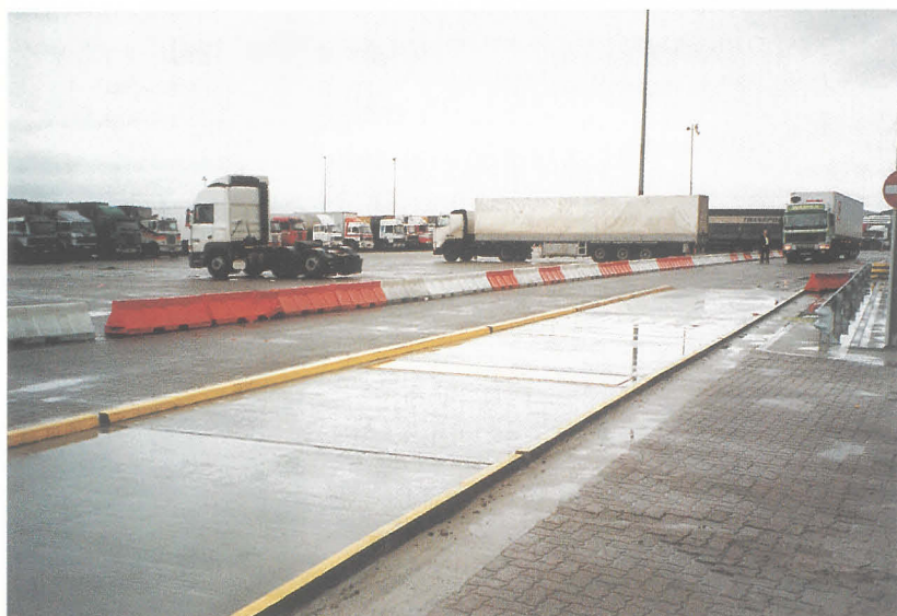
Fig. 1 General view of an integrated dynamic axle weigher. A single-axle load receptor is situated on the apron; the latter serves to minimize level variations since a flat weighing zone is vital to obtain good performances in this type of measurement.
