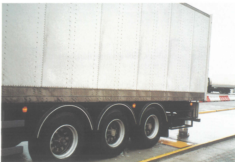
Fig. 2 Different types of European vehicles that can be weighed - transfers of load within compensated axle systems constitute an important factor relating to the achievable accuracy of WIM systems.
