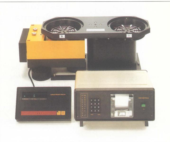
Fig. 2 Fully automatic mass comparator for testing mass standards up to 10 kg.
