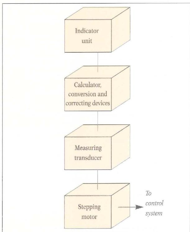
Fig. 2 Subsystem of the fuel dispenser
