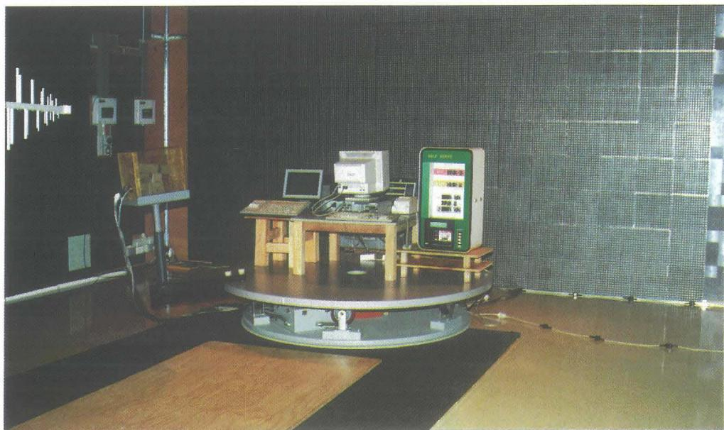
Fig. 3b Stepper motor system in NSC's chamber
