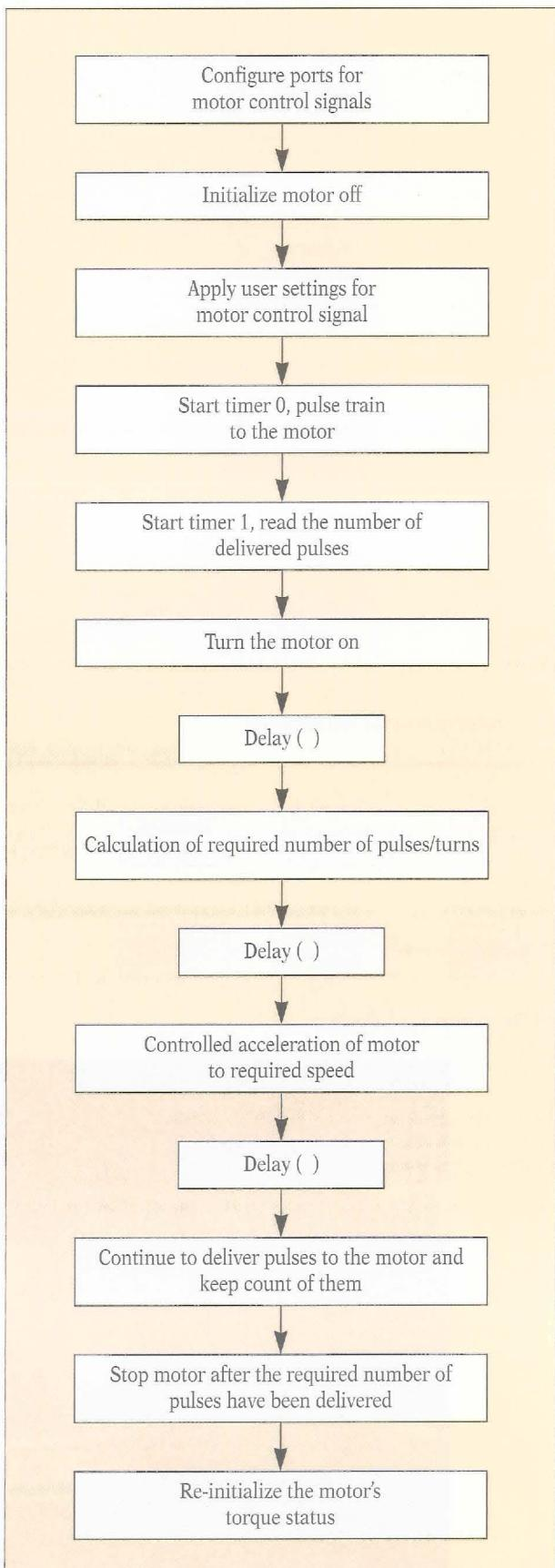
Fig. 4 Flow diagram of the stepper motor program
