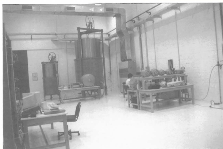
Fig. 2 Low flow rate gas facilities: the two bell provers are shown just behind the bench of wet test meters.
