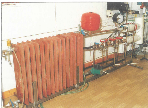
Fig. 2 The first experimental apparatus for energy metering
