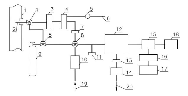
Figure 1 - Example of the composition of a gas analytical system using calibration gas mixtures for its adjustment (for illustrative purpose only)
