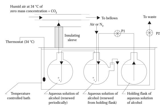
N.B.: Pumps P1 and P2 have an identical flowrate of approximately 0.33 L/h
