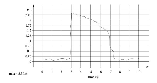
Example of the curve of the flow rate as a function of time, as obtained from a test rig (see 5.1)
