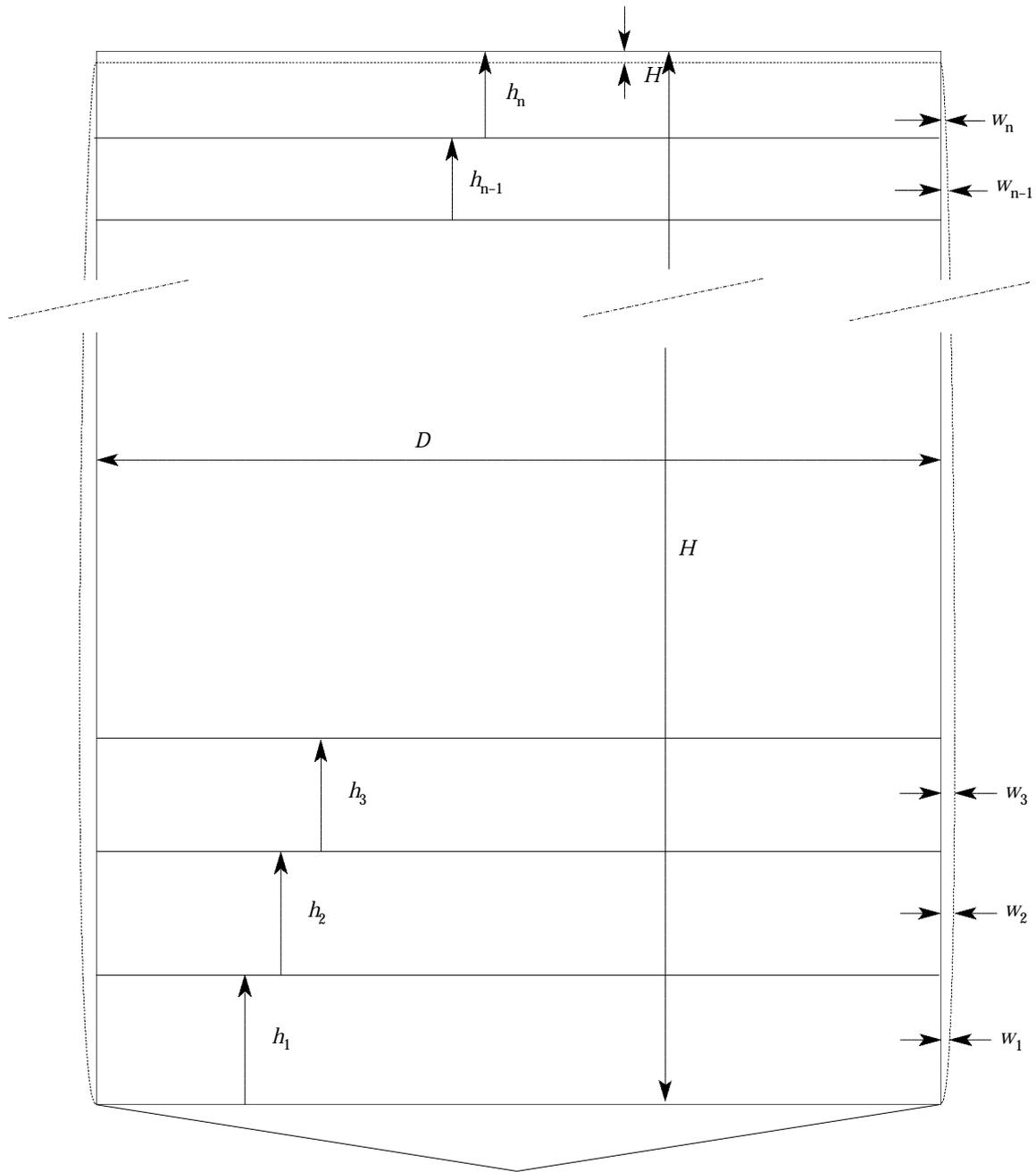
Figure 2 Deformation of tanks
