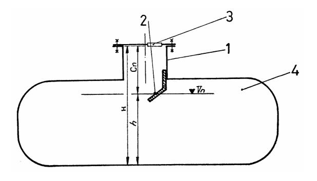
Fig. A.4 Single volumetric mark in tank (on console fixed to dome)
