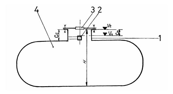
Fig. A.1 Single or two (opposite) volumetric marks or indexes in the dome
