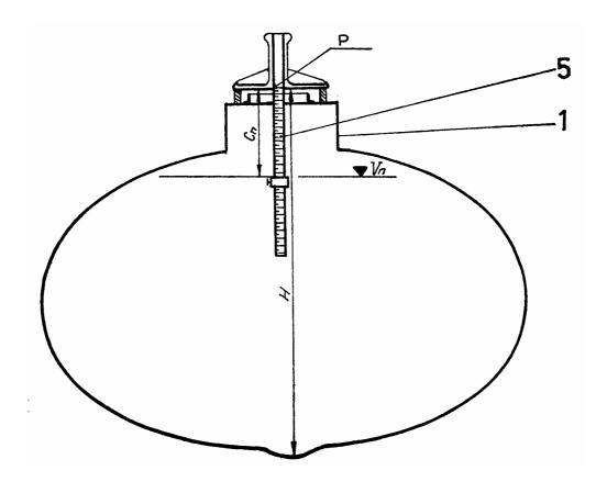
Fig. A.5 Mechanical dipstick with sliding index
