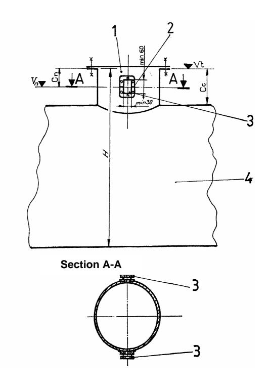
Fig. A.3 Single mark or graduated window in dome
