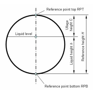
Fig. 1 Schematic view of a tank to determine 2.15 - 2.19
