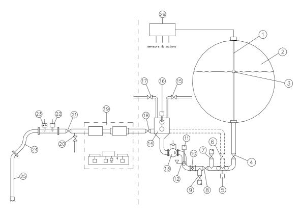
Fig. B.2 Schematic setup of the measuring system of a road tanker for milk in its maximum version (for explaining the basic components and functions)
