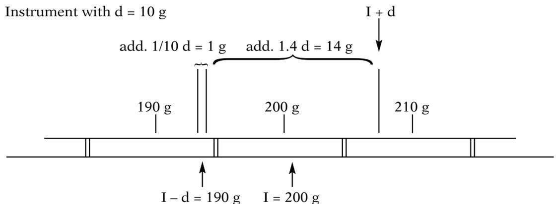
The indication at the start is  $I = 200 \text{ g}$ . Remove additional weights until the indication changes to  $I - d = 190 \text{ g}$ . Add  $1/10 d = 1 \text{ g}$  and thereafter  $1.4 d = 14 \text{ g}$ . The indication shall then be  $I + d = 210 \text{ g}$ .
