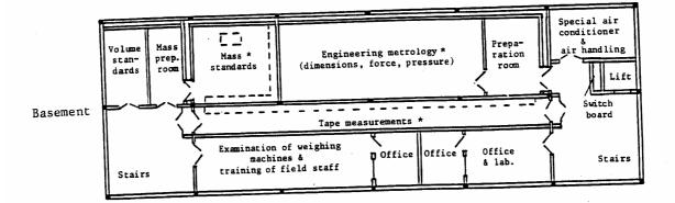
Fig. 4 - EXAMPLE OF LAY-OUT OF MAIN METROLOGY BUILDING
