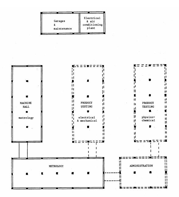
Fig. 2 - PRACTICAL LAY-OUT OF THE METROLOGY BUILDINGS WITH POSSIBLE EXTENSION FOR PRODUCT TESTING
