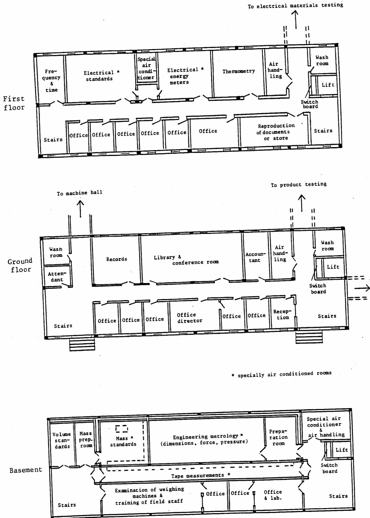
Fig. 4 - EXAMPLE OF LAY-OUT OF MAIN METROLOGY BUILDING
