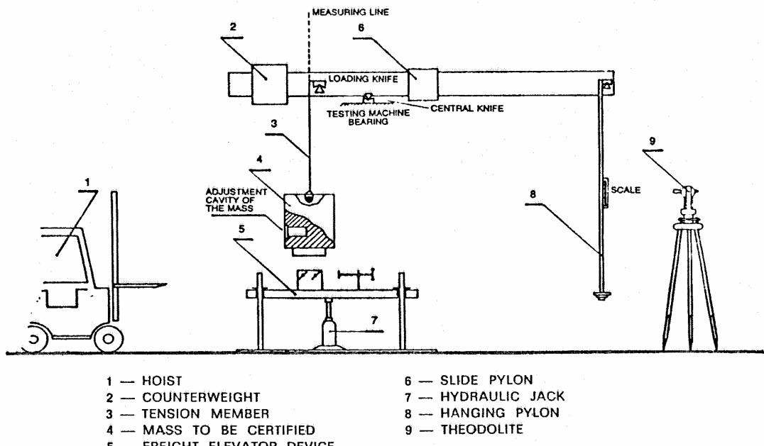
A mechanical mass comparator constructed at INIMET for the verification of 1000 kg mass standards and described in INIMET Scientific-Technical Bulletin 1-1986
