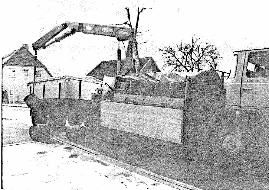
Tracting lorry with three axles, distance between extreme axles 3.8 m, total admissible weight loaded 22 t, unloaded 12.5 t. Crane at the rear, capacity 110 kN·m with external jack stabilizers.
