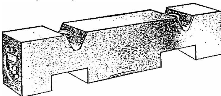
Fig. 1 — 1 000 kg block weight Length 1
