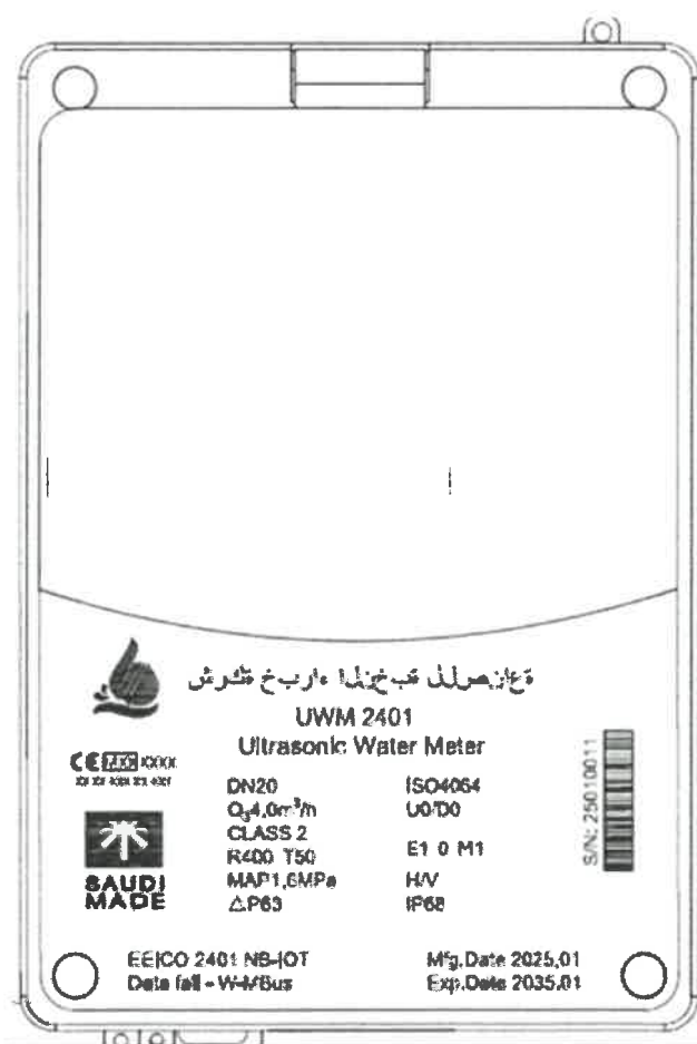
Fig. 1: Illustrative view of the water meter type UWM 2401
