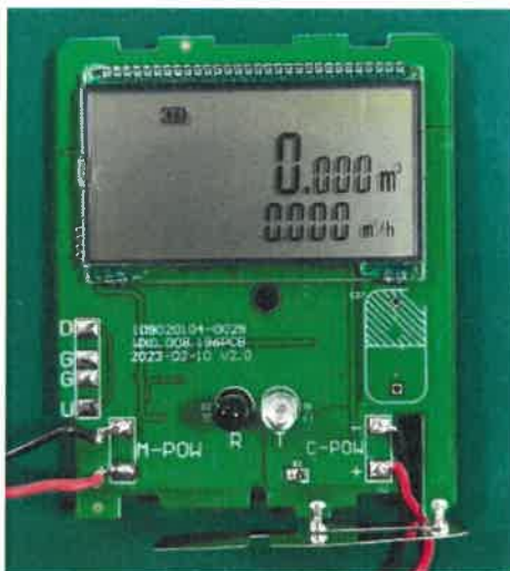
Fig. 7: PCBA photos of water meters U-WR2 series
