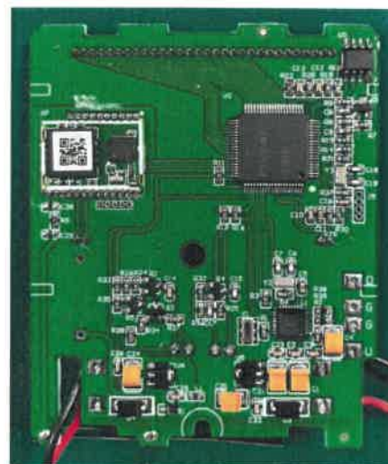
Fig. 7: PCBA photos of water meters U-WR2 series
