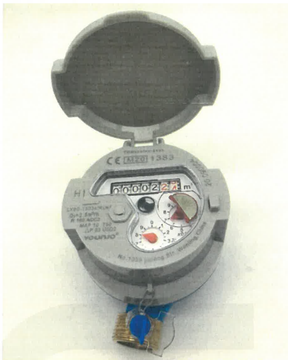
Figure 3: The water meter type LXSG-xxD3n/RLN1 – view and sealing
