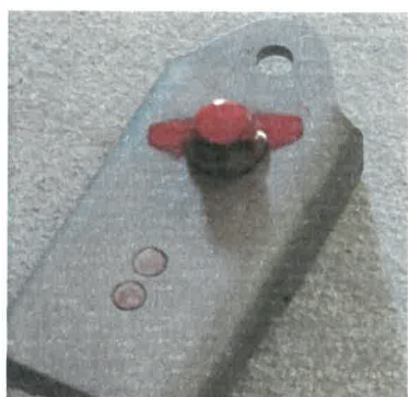
Figure 2 Anti-tamper paint on the sensor
