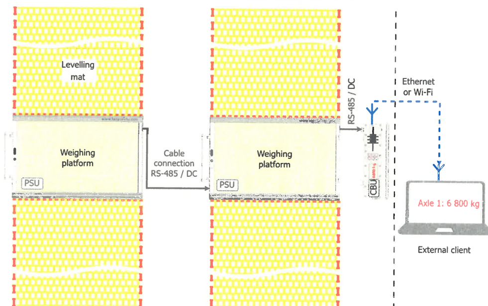
Figure 3: Configuration with a pair of platforms communicating via cable over the RS-485 bus with the Indication unit. The Indication unit may communicate further with external SW clients via Ethernet or Wi-Fi interface.
