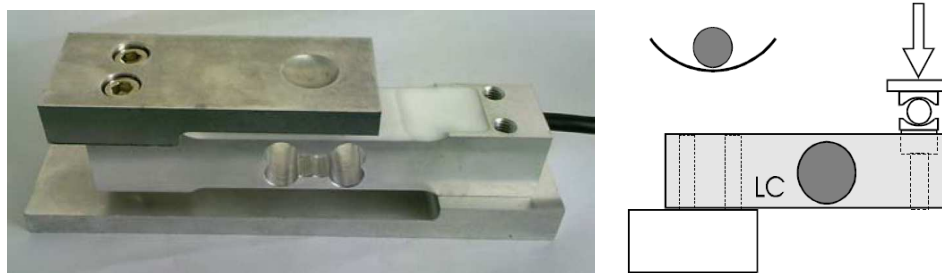
Figure 3: Examples for a force introduction of the load cell type ERS
